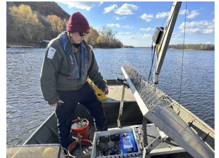
Minnesota DNR Invasive Carp Field Lead Kayla Stampfle inspects the components of a telemetry receiver that tracks tagged invasive carp in the Mississippi River near La Crosse. The solar-powered receiver can transmit real-time notifications of the movements of tagged invasive carp.
