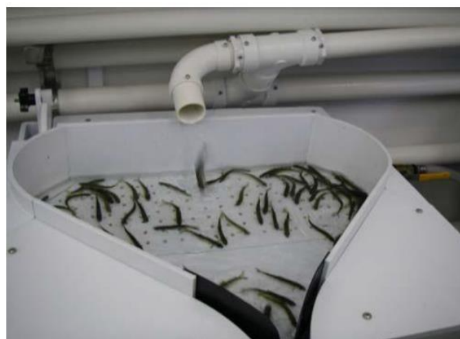
Fish are sorted by size and moved through an automated system within each trailer where they receive an adipose fin clip and a coded wire tag.
