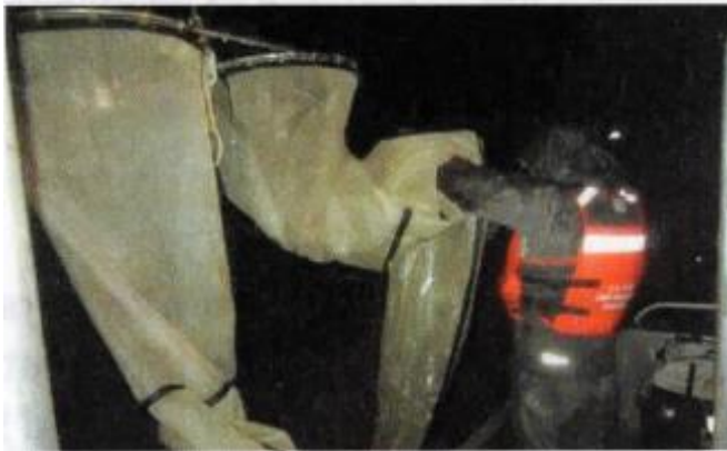
Bongo nets are used to sample the ichthyoplankton community as part of the Early Detection Program.
