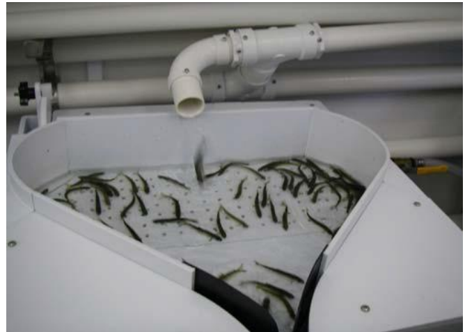
Fish are sorted by size and moved through an automated system within each trailer where they receive an adipose fin clip and a coded wire tag.
